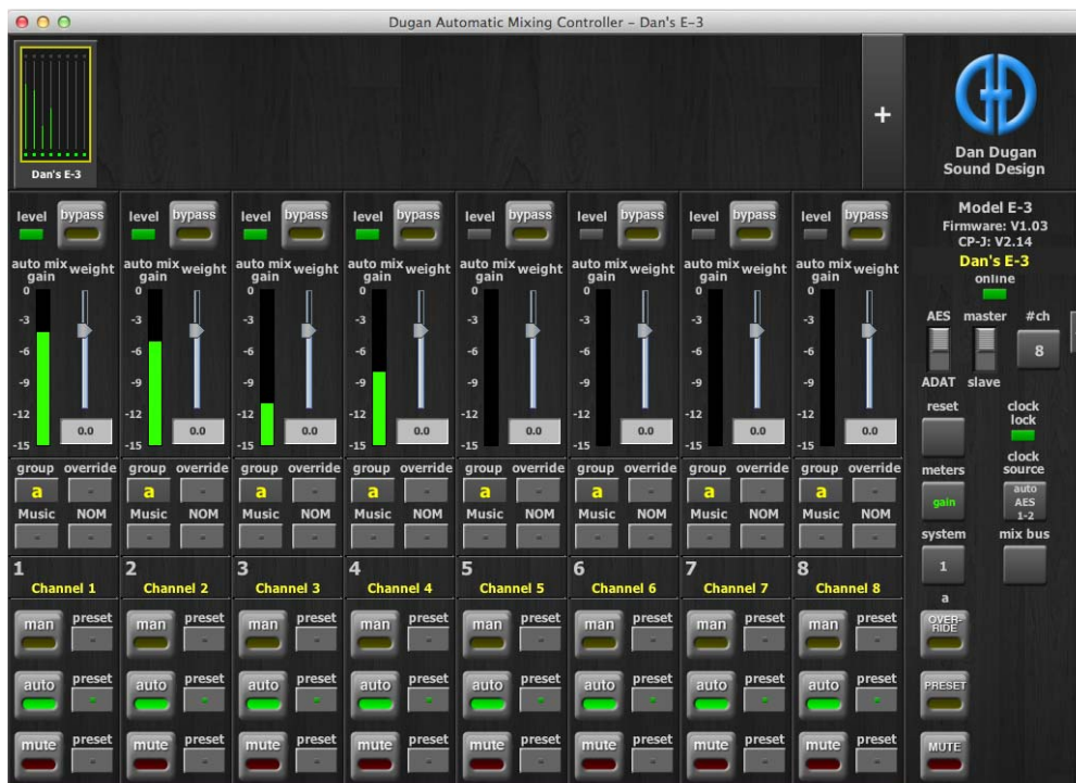
Figure 5-1 Dugan Control Panel
