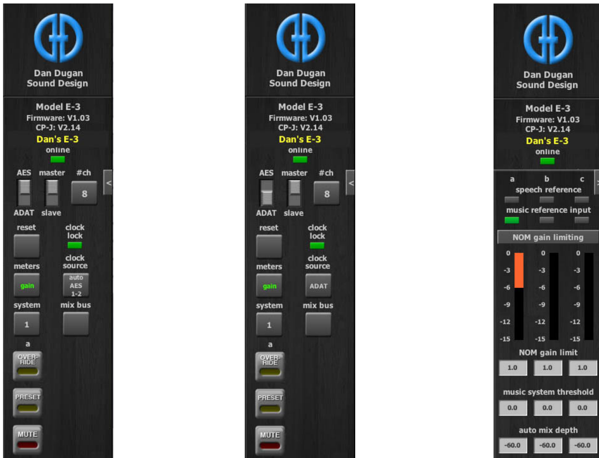
Figure 5-11 Master Pane: AES settings (left), ADAT settings (center), Music System controls (right)
