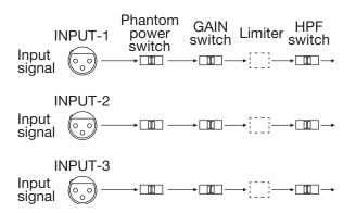
Set the following switches and control for each input channel to match the input source.
