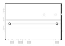
On each of the left and right sides of the bracket, there are three holes for inserting the screw for fixing the bracket to the unit. Depending on which hole you choose, you can adjust the DSLR position back and forth.
