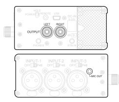
The [OUTPUT] jacks are normally connected to an external mixer, recorder or amplifier.
