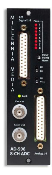
**DB25 Connectors** conform to the Tascam pin out. Please note you can't use a pin to pin DB25 cable to connect the digital outputs to a DB25 digital input connector. A special cross cable is required.
